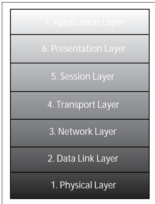
Figure 3.1 The OSI model separates networking functions into seven layers.
